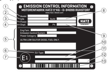
The layout of the EPA/CARB type plate depends on the engine application and is affixed to the crankcase.
